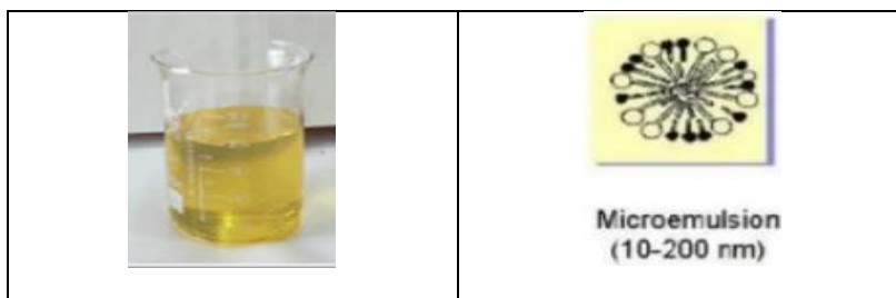
Figure 3: Microemulsion formulation, ME (Left), Micelle size (Right)
